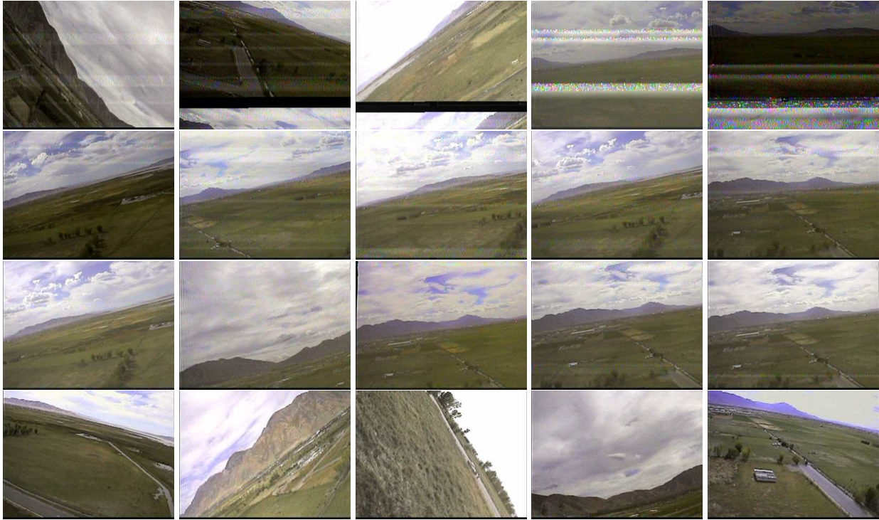
Figure 4: Wireless video classification examples. Each row shows five examples of a classification result within a given prediction range. (Row 1) Noisy: 0.95-1.0 (Row 2) Slightly noisy: 0.5-0.95 (Row 3) Clean: 0.05-0.5 (Row 4) Very clean: 0-0.05. These results show that the classifier predictions qualitatively match human intuition about "noisy" and "clean" as the noise gets lower and the prediction approaches zero.
